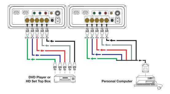
Figure 3-11. RGB Connections
